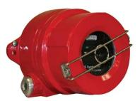
A high-speed microprocessor based fire detection and process control system specially designed for liquid and powder coating applications, the FS System 10<sup>™</sup> quickly detects the presence of a flame, reacts by initiating a shutdown of the electrostatic finishing process in a matter of milliseconds: and effectively interrupts the fire before residues and wet paint films can ignite.
