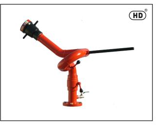
The monitor has large flow capability and can be manually operated by a single fire fighter. The design ensures to prevent jet reaction forces from effecting the horizontal and the vertical position of the monitor. The counter balance is not required to offset the weight of the nozzle. The monitor has the ability for 360 deg. continuous horizontal rotation and angle of elevation from +90 deg. above horizontal and 45 deg. below horizontal.
