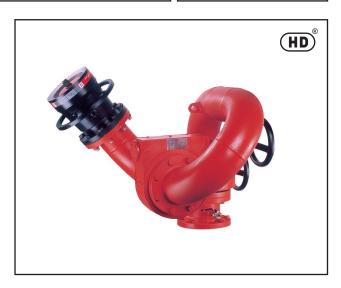
The monitor has large flow capability and can be manually operated by a single fire fighter. The design ensures to prevent jet reaction forces from effecting the horizontal and vertical position of the monitor. The monitor has the ability for 360 deg. continuous horizontal rotation and angle of elevation is adjustable with fix stop from 90 deg. above horizontal to 65 deg. below horizontal.
