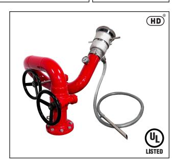
The Monitor has welded Stainless Steel 4 inch (100mm) waterway. Vertical and horizontal rotation is through stainless steel swivel joints with double row of stainless steel ball bearings. Both vertical and horizontal movements are controlled with handwheel driven enclosed worm gear.
